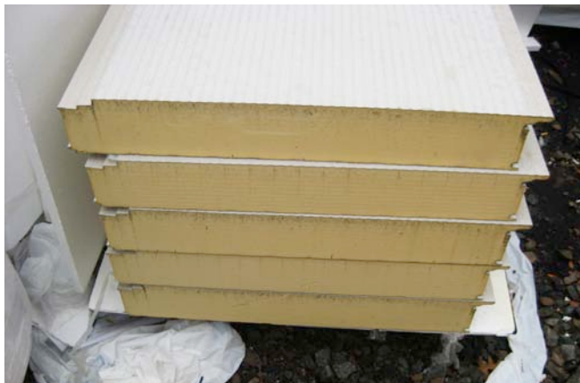
Photograph 3: Insulated Metal Wall Panels —The upward “tongue” of the lower panel functions similarly to the elevated vertical leg of a “metal flashing”.
