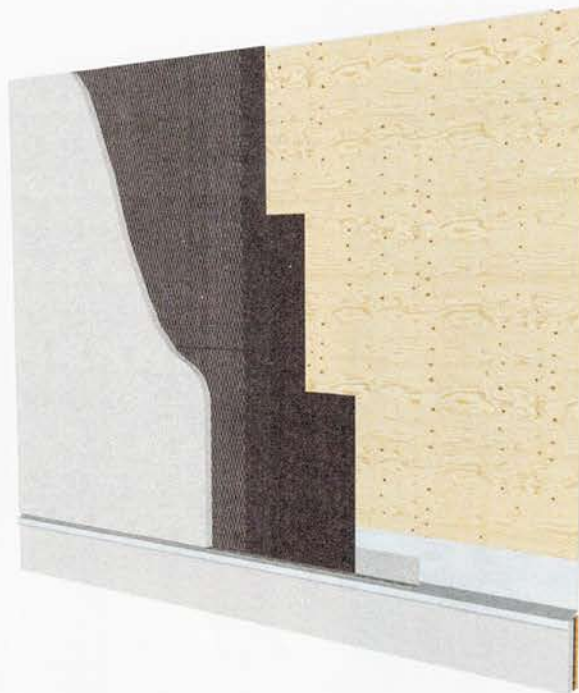
Stucco is commonly installed over wood framing with plywood sheathing or steel framing with gypsum sheathing back-up walls. Stucco is arguably low maintenance and adaptable to both classical and modern architectural styles.
